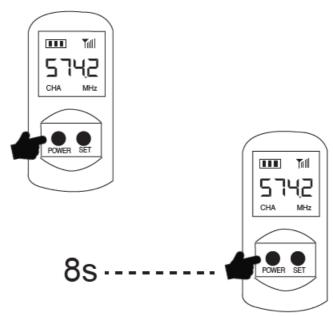
2. Long press the power button for 8 seconds to change channel.
