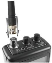
2. Press the antenna over the jack and turn the base of the antenna clockwise to secure it.
