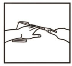
6. First keep the knife away from you and keep your right hand close to the stone. Keep the guide on the stone to get the perfect 18 degree angle. Pull the knife toward you while sliding it to the right. Repeat 4-5 times go back to step 5 until satisfied.
