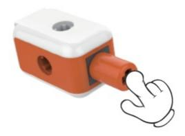
**Touch sensor:** When the button is pressed, it transmits information to the host for controlling subsequent programs. In the program, it is generally used as a judgment condition in wait until command or repeat until command.
