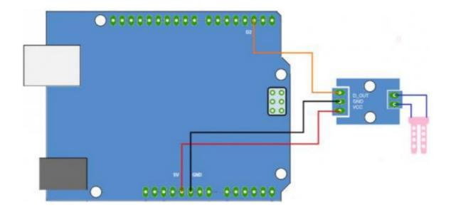
The water level sensor gives an analog voltage corresponding to the water level present on the sensing element. If a larger proportion of the sensing elements are exposed to water, the output voltage will increase.
