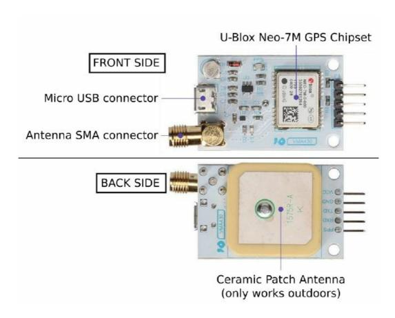
The NEO-7 series of standalone GNSS modules is built on the exceptional performance of the u-blox 7 GNSS (GPS, GLONASS, QZSS and SBAS) engine. The NEO-7 series delivers high sensitivity and minimal acquisition times in the industry-proven NEO form factor.
