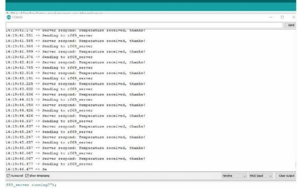
3. Open a new IDE with the RF69\_SERVER\_RECEIVE\_DATA code and upload to the Arduino® without the temperature sensor. You should see following output:
