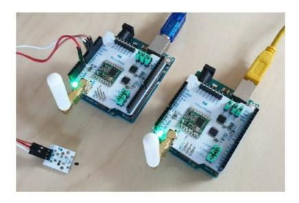
We will connect two radio shields to one another, read the temperature and send the temperature value to another module. Requirements:
