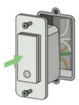
Screw the Dimmer into the wall. Be careful not to overtighten the screws.
