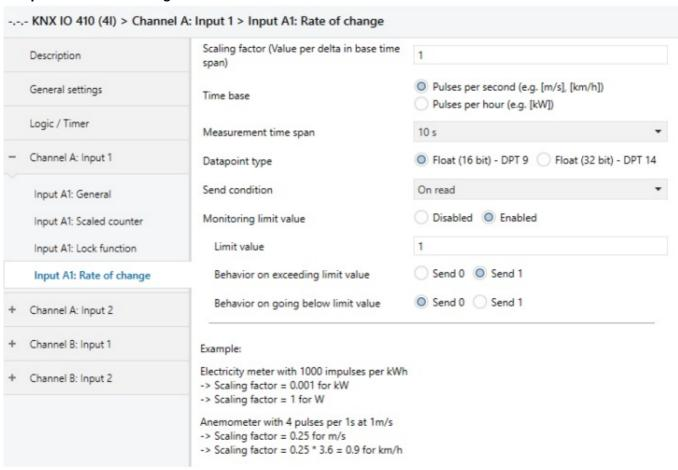
This counter is used to connect devices to the bus where the rate of change is critical within a time interval, e.g. an anemometer.
