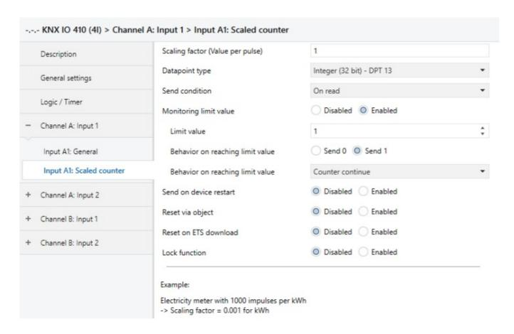
This counter can be used to count values on input impulses, where an integer value or a floating-point value can be selected as a counter variable. With this function, e.g. Electrical energy can be counted directly and sent to the bus via an object.
