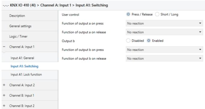
If the switching function is selected, up to 2 binary switching telegrams can be sent via the following objects:
