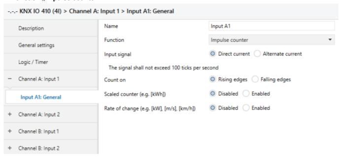
If the impulse counter function is selected, further parameters are displayed in the general settings of the input channel. Here, the general settings of the impulse counter are made, a scaled counter and/or counter of the rate of change must also be selected.
