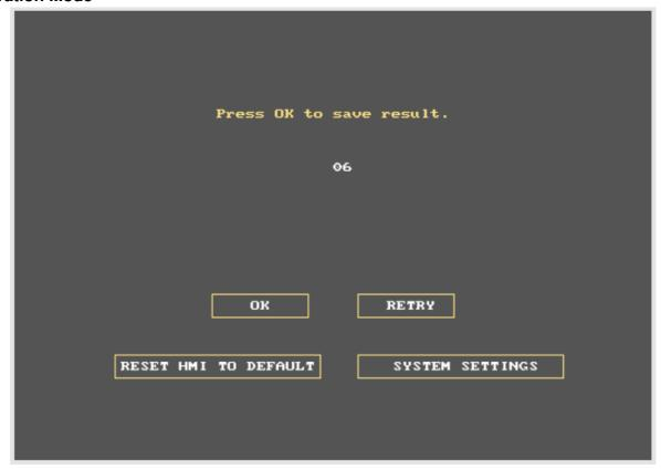
Press and hold anywhere on the screen when HMI starts until it enters touchscreen calibration mode. If "Enable [Reset HMI to default] button in calibration mode" is selected as described in Part 5 System Settings, then [RESET HMI TO DEFAULT] and [SYSTEM SETTINGS] buttons can be found in calibration mode. Follow the onscreen guide and press [yes] to restore factory default, and please note that the projects and data stored in the unit will all be cleared after this.
