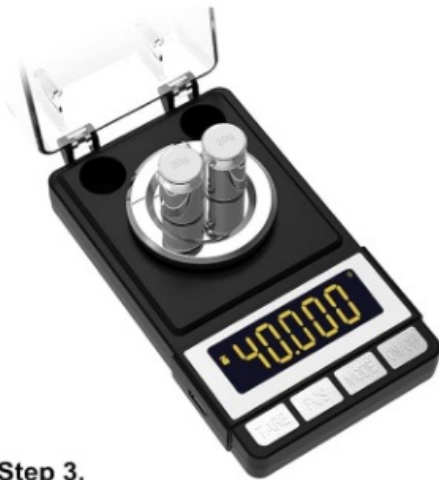
Step 3. The display starts to flash 40.000, Place another 20g calibration weight on platform
