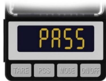
Step 4. "PASS" shows on screen, then remove the calibration weight from the platform
