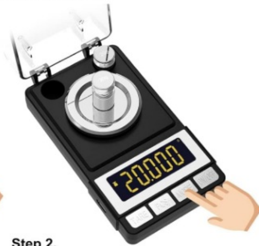
Step 2. Press "MODE" key for 6+ seconds, until the display starts to flash 20.000, Place 20g calibration weight on platform
