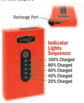
It takes 2.5 hours to fully charge when using a 2.1A USB adapter. The power indicator lights will flash one by one while the unit is charging. A solid light indicates a completed level of charge, while a blinking light means the
