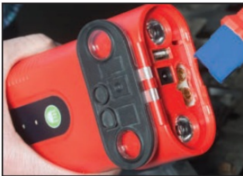
Once it Starts, Disconnect Clamps from Weego 70
