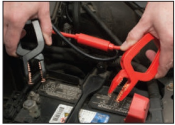
Detach Clamps From Battery
