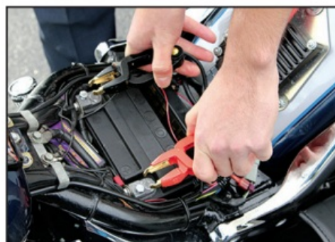
Detach Clamps From Battery
