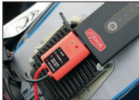
When You Have GREEN LIGHT On Your Smart Box, Start Your Engine
