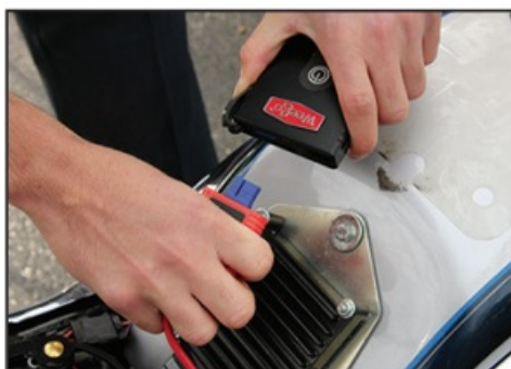
Once it Starts, Disconnect Clamps from Weego 22
