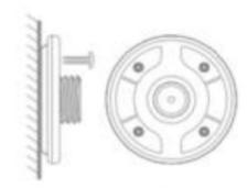
3- Rotate and close the top cover of the base and install the equipment
