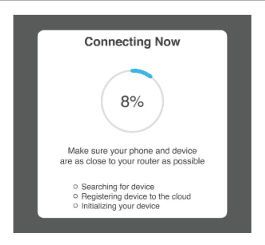
STEP 4: The app will try to connect your device. During this time, the camera will beep, start quickly bli nking Red, and then turn solid Green.
