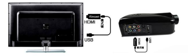
**Note:** pls check whether the USB Port of the TV or projector is workable or not. If not, please use the USB cable to connect the USB power adapter to charge the wecast wireless display receiver.
