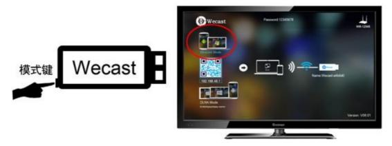
Open the android device's wifi, then come to the screen share menu to Select Wecast wireless display receiver SSID Wecast – XXXXX and connect to the Miracast function as follows:
