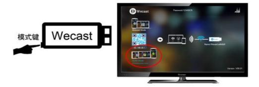
The iOS devices airplay and airplay mirroring function setting Open the WIFI of the iOS devices, search and connect to Wecast wireless display receiver SSID wecast – XXXXX (the default password: 12345678), back to the desktop, upper the home screen menu of iOS devices, Enter into airplay mode and press Airplay or airplay mirroring function to cast or mirror the local video, audio, image, and online video from iOS devices to TV or projector.
