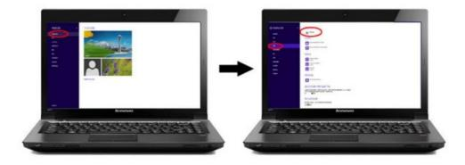
The system will automatically search Wecast wireless display receiver SSID wecastxxxx, press it, and then wait for connection.
