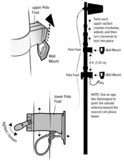
Clean surface of RV where wall mounts will attach and remove the **adhesive backer** on both the upper and lower wall mounts.
