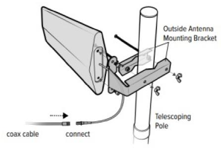
STEP 2 Mount Telescoping Pole to Side of RV
