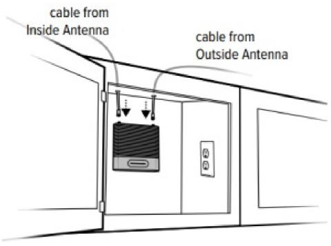
Connect AC power supply to end of booster labeled "
