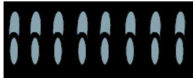
(C) Soft blue flames: Normal for Natural Gas
