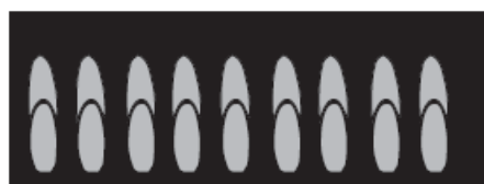
(A) Soft blue flames— Normal for natural gas
