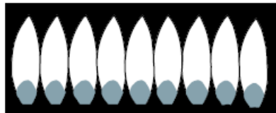
(A) Yellow flames: Further Adjustment Required
