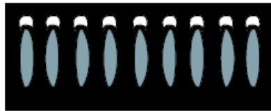
(B) Yellow tips on outer cones: Normal for Propane Gas
