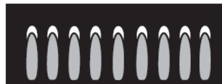
(B) Yellow tips on outer cones— Normal for propane gas
