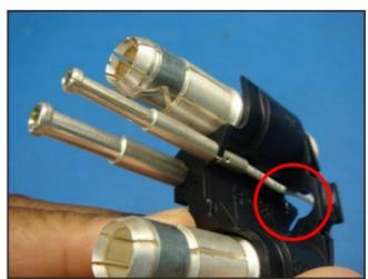
5. Re-insert the contacts assembly into the main connector housing and snap it into position to lock it into place.
