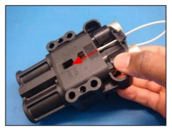
6. Confirm the contacts are inserted in the proper locations as shown.
