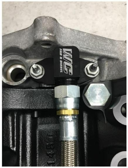
6. On 2001-2010 models, the OEM turbo feed line is in the valley center of the block. You will install the supplied m12 fitting here to block this port.
