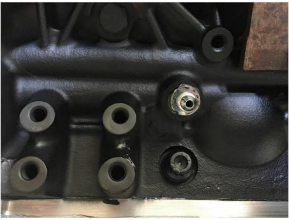
4. Next locate the 1/4" NPT X #4 JIC straight fitting. Apply Teflon Paste (DO NOT use teflon tape!) to the threads
