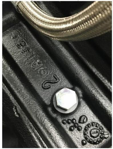
7. Next locate the billet turbo drain flange. The drain flange can be installed on the turbo center section with the supplied Allen head or hex head flange bolts and gasket as shown.
