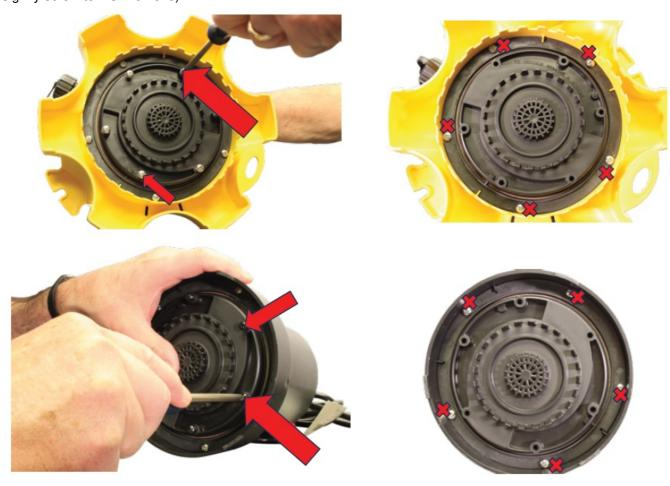
4. Using care to not tear the cork gasket on the bottom side of the inlet screen, gently separate the inlet screen from the pump. Clean and rinse any debris from the inlet screen.
