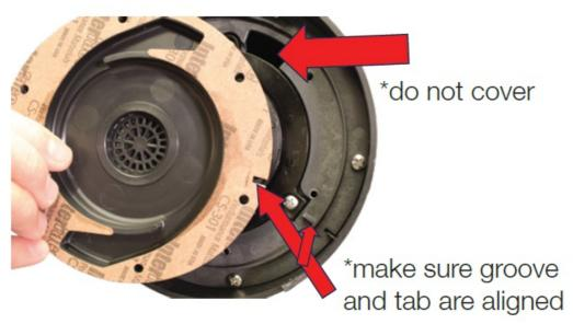
7. Reinstall the inlet screen using caution not to over tighten or strip the screws or screw holes.
