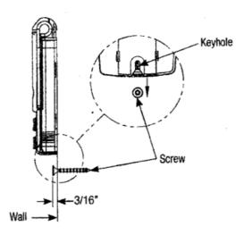
If mounting to a NEMA electrical device box use machine thread screws provided in place of the wood screws. No drilling is required. If high voltage wiring is contained in the box a standard NEMA solid faceplate must be installed between the box and the wall station.
