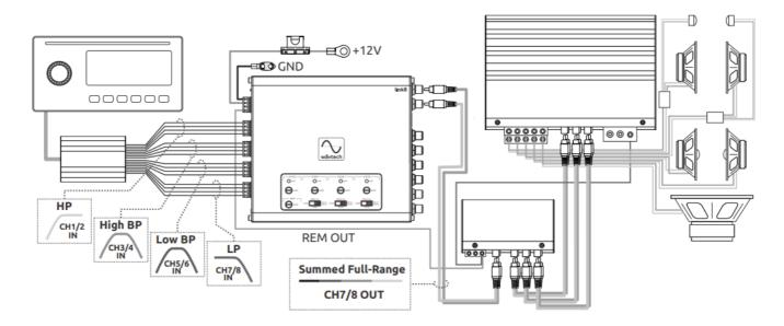
**Note:** For systems where no full-range signal is available, the link8 can be utilized purely as a 4-way summing line output converter without remote. In this example, the link8 is summing factory 4-way signals to a single pair of 2-channel full-range outputs so can be altered by aftermarket crossover, processor or amplifier(s) that is not capable of summing.
