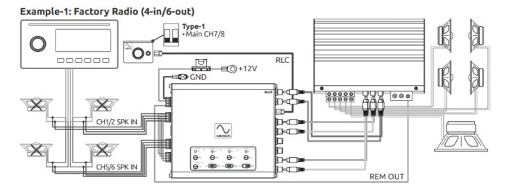
**Note:** For systems where only remote sub-level control is needed for a speaker-level source, select system Type-1 (factory setting) at the multi-function remote. For a 4-channel source as shown above, multiple input configurations can be chosen with the link8. This particular 5-channel aftermarket system could benefit from retaining front/rear fading as well as a
