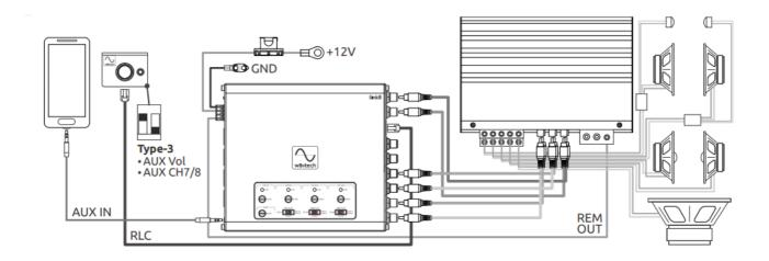
**Note:** For stand-alone systems where only the AUX input is used, select system Type-3 at the multi-function remote. This disables the remote's source select function and sets knob priority to master volume control for AUX input. Portable devices such as smartphones or MP3 players typically have an output voltage of 1Vrms or less, so it is recommended to maximize the device's unclipped output level and use the remote for the system's master volume.
