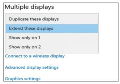
3. Scroll down to the "Multiple displays", and select the mode in the drop-down list that is fit for your need.
