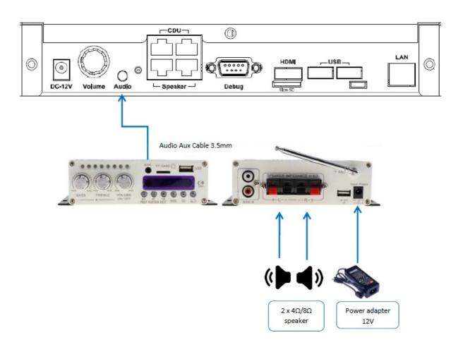
Wiring Diagram with whole system
