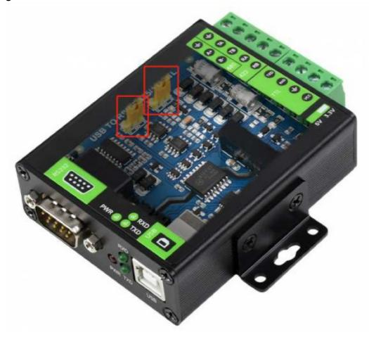
**Note**: The RS422 and RS485 interfaces of USB TO RS232/485/422/TTL also have a built-in 120R enable resistor, which is enabled by default, and the user can disassemble the case to modify the settings as needed. Modification method: modify the yellow jumper cap at the red frame.
