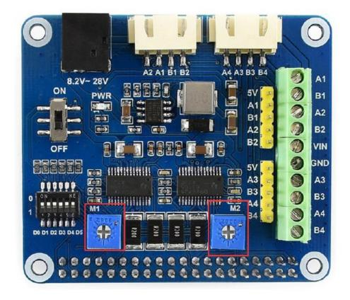
Generally, working current of stepper motor is less than 2.5A, in this case, we need to adjust the current outputted.
