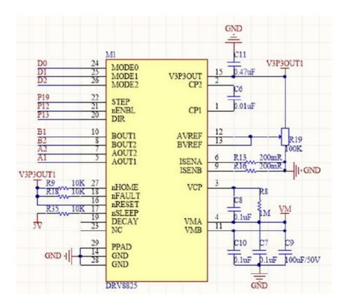
The DRV8825 is e has two H-bridge and a microstepping indexer, and is intended to drive a bipolar stepper motor. It supports up to 1/32 microstepping. Internal shutdown functions are provided for overcurrent, short circuit, under voltage lockout and over temperature.
