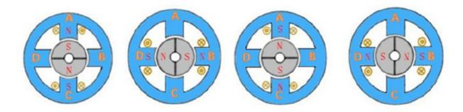
According to Ampère's circuital law, when current of coil A flow from left to right, stator generates magnetic field, internal side is North pole which will adopt rotator of motor. When the currents of four coils based on certain rule, they will generate a rotate magnetic field and drive the rotator rotate. If every motor has four rotators, it has four statuses:
