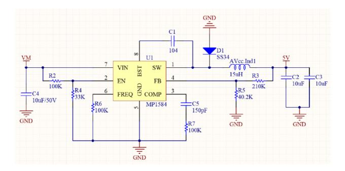
MP1584 regular supports wide 4.5V to 28V input, and up to 2A current output. Even thought that MP1584 support low to 4.5V input, however, VM also supply power for motor controller, which require at least 8.2V. So, the recommend input voltage is 8.2~28v.
