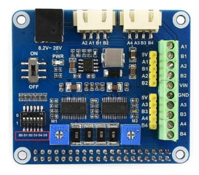
D0, D1, D2 are used to control motor M1 (MODW0, MODE1, MODE2), D3, D4, D5 are used to control motor M2 (MODE0, MDOE1, MODE2). Their relationship are as below:
