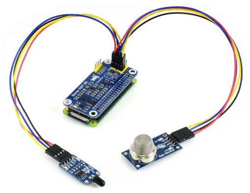
• Connect to Raspberry Pi 4 (requires a pin header )
