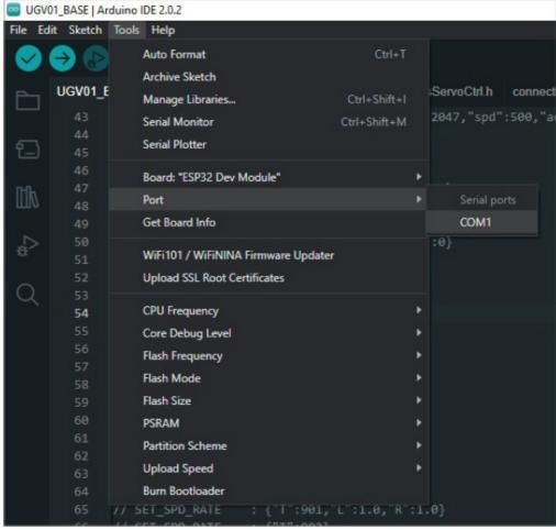
4. Connect the driver board to the computer with a USB cable, then click Tools – > Ports, select uf2 Board for the first connection, and after the upload is complete, connecting again will result in an additional COM port.
