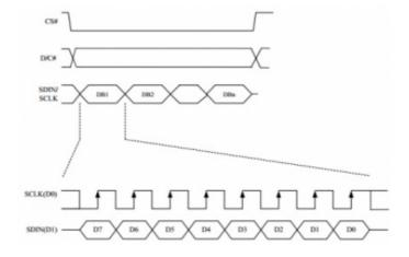
Since the ink screen only needs to be displayed, the data cable (MISO) sent from the machine and received by the host is hidden here.
