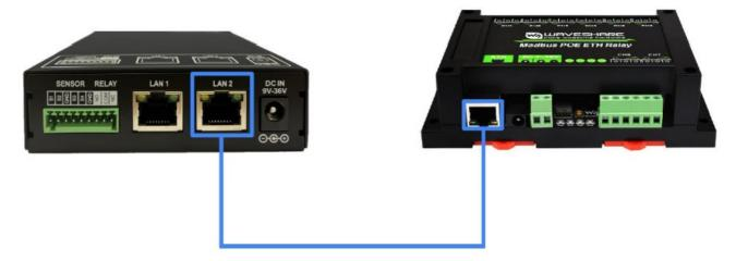
You will connect the Relay to LAN1 for use. It must be used after setting up the router. If the router is not POE-enabled, you will need to supply additional power to the Relay and change its IP address. Since the Relay is an external device, this use case is not recommended due to security concerns.
