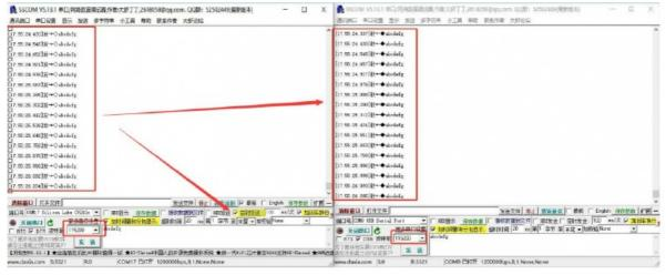
3. Then check the timing sending in the right window, and the time can be set to 100ms/time to see if it is sent to the left window normally, there will be no packet loss or garbled characters, and if it is normal, turn off timing sending, as shown in the figure below:
