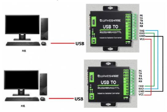
2. Open two sscom software windows, open the corresponding serial port number, set the baud rate to 115200bps, enter the box "abcdefg", then open the serial port, and perform the sending and receiving test: (the
