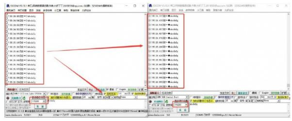
3. Then check the timing sending in the right window, the time can be set to 100ms/time, and see if it is sent to the left window normally, there will be no packet loss or garbled characters, and if it is normal, turn off timing sending, as shown in the figure below:
