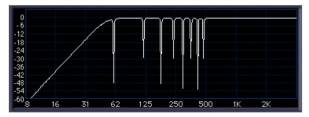
The graph represents the X-Hum notch filter settings. The x-axis shows frequencies in the range 10 Hz - 4 kHz (logarithmic scale). The y-axis shows amplitude from +6 dB to -60 dB.
