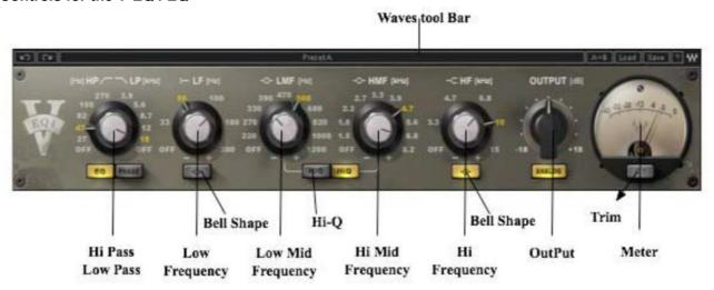
As with the V-EQ3 EQ, you can select a frequency by clicking the desired location on a knob. The inner knob sets the gain for a filter, while the outer ring is used to set the frequency. Click on a desired frequency to select that value, then drag to a gain value, which is continuously variable. If you prefer, you can enter values numerically by
