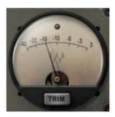
Measures the output peak of the EQ device, measured in dBFS. Click on the trim button to reset the output of the EQ to -0.1 dBFS. A red clip light indicates over-level. It can be reset by clicking on it.
