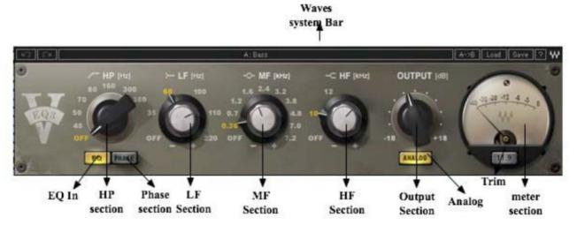
Unlike most Waves plug-ins, the V-Series plug-ins do not display frequency, gain, or other parameters in Value Windows. In keeping with the vintage feel and sound of these tools, values can be read from the knob positions on the interface. The LF, MF and HF (LP, LMF, HMF and HP in the case of the V-EQ4) controllers are double knobs. The inner knob controls gain and the outer ring sets the cutoff frequency.
