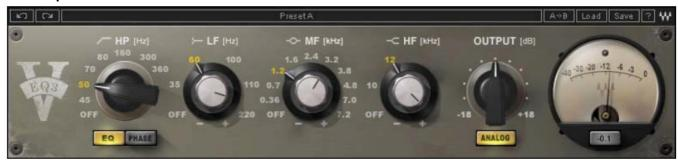
The Waves V-EQ3 Equalizer is three-band EQ with a highpass filter. Like the 1073 and 1066 hardware devices after which it was modeled, the V-EQ3 offers selected cutoff points and  $\pm 18$  dB gain adjustment with a bell-shaped curve. The highpass filter can range from off to 360 Hz, with a slope of -18 dB per octave. Output gain can be adjusted up to  $\pm 18$  dB.
