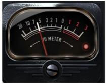
Use the screwhead to calibrate the meter to your DAW reference. Range: -12 dB to +12 dB
