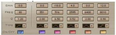
Each band in the LinEQ has a band strip with 5 controls that define the settings
