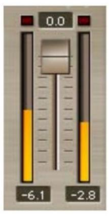
The Output meters and clip lights show the output energy in the Left and Right channels in dB from 0dB down to – 30dB. The clip lights light up together when any output clipping occurs. A peak hold indicator under the meters shows the peak value until reset by clicking on it.
