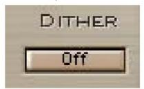
As the LinEQ process is a double precision 48bit process, the output is rounded back to 24bits. While the equalization doesn't present quantization error and noise, the rounding back to the 24th bit may. It is On by default, but it is the choice of the engineer weather to add low level hiss like noise or to get slight low level nonlinear distortion from quantization noise. Either noise types will be extremely low and rather inaudible.
