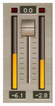
The gain fader lets you reduce the Signal's gain. When you apply strong peaking EQ, overriding the full digital scale will cause distortion. If your signal is hot and you want to boost some of it further, the gain fader lets you get more manipulation headroom. Using the auto Trim control can also set this gain value for accurate compensation of over full scale values.
