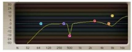
The EQ graph shows a view of the current EQ settings. It shows Frequency at the X axis, and Amplitude t the Y axis. It also provides a visual work surface. Setting EQ parameters directly on the graph is possible by click dragging each of the 6 band's grab markers. Alt-Drag would change the Q for the selected band and Ctrl-Click would toggle the Type. The graph has 2 possible amplitude scales showing either +/-30dB or +/-12dB.
