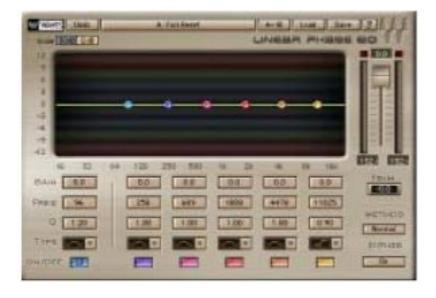
This is the main broadband component offering 6 Linear Phase EQ bands. Band 0 or LF is the Low Frequency Band and it offers a range from 22Hz to 1kHz with 1 Hz resolution for precise low frequency cutoffs. The other 5 bands work in frequencies 258Hz – 18kHz. The resolution is 87Hz and intended mostly for the higher frequencies.
