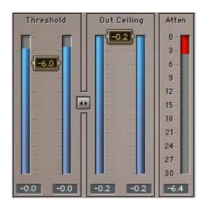
**THRESHOLD:** 0.0 to -30dBfs, Default 0. The Threshold value sets the point that the audio energy should be limited to. When the energy goes over the Threshold, Gain attenuation will be applied to keep it just below the Threshold. The L3 will also add make up Gain in an opposite value to the Threshold.
