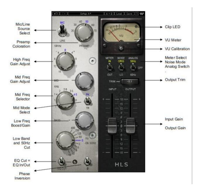
**3.2 Controls Source Select** toggles between Mic and Line levels.
