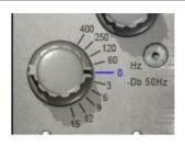
**LF Selection** (upper half) 0 (Off) to 400 (60, 120, 25 Hz) **50 Hz Attenuation** (lower half) 0 (Off) to 15 (-3, -6, -9 15 dB) **Default** 0 (Off)
