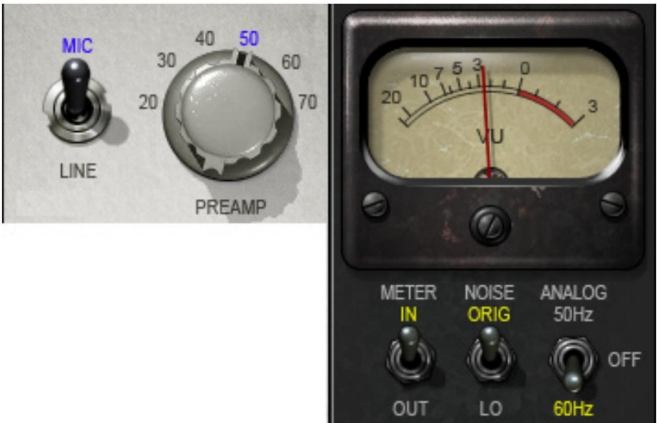
If the noise level is excessive, set the Noise switch to LO. To retain only the modeled harmonic distortion, bypass the noise and hum by setting Analog to OFF.
