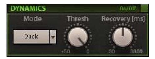
This section allows you to apply compression to the wet path, that is, to compress the reverb tail using a detector on the wet path itself or on the dry path,
