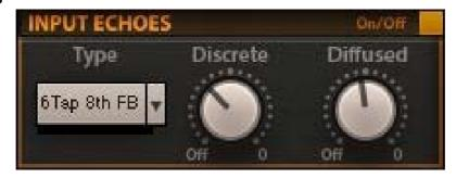
The Input Echoes section replicates the input audio using up to 6 delayed taps which can be fed discretely to the effect's output or into the reverb generator.
