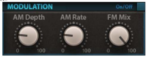
To add even more fun to the game, we've included some modulations. You can add some stereo sensation by applying amplitude modulation on the input to the reverb effect. You can also add some magic by mixing subtle frequency-modulated (pitch-modulated) replica at the output. To hear the effect most pronouncedly, you can play a continuously sustained note and play with the controls.
