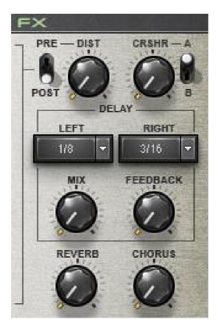
**DIST** controls the amount of distortion effect. Distortion is applied per voice, eliminating IMD (inter-modulation distortion.) Settings below 50% create a warm saturated drive effect; settings above 50% result in a more aggressive, "crunchier" sound.
