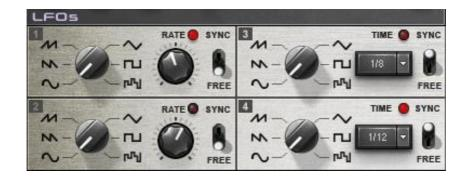
Element 2.0 features four identical LFOs that can be either free-running or synced to both MIDI clock and Note On commands.
