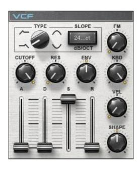
The VCF section includes selectable filter slope, frequency and resonance parameters as well as a filter envelope which determines the filter movement on each trigger.
