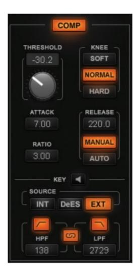
COMP: Turns on or bypasses the Compressor section.
