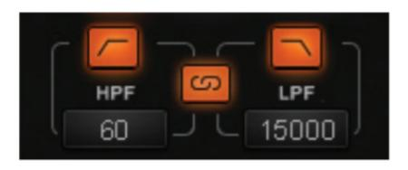
In addition, the Key signal (whether internal or external) can be filtered using HP/LP filters.
