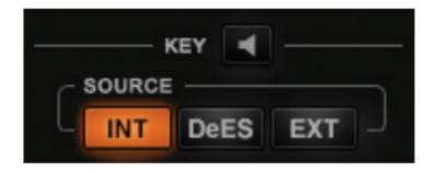
The Key feature adds additional precision in controlling dynamics. The Key acts as a trigger that activates the dynamic process. The Key can be internal – triggered by its own signal, or External – triggered by another audio channel through sidechain routing to the Compressor.
