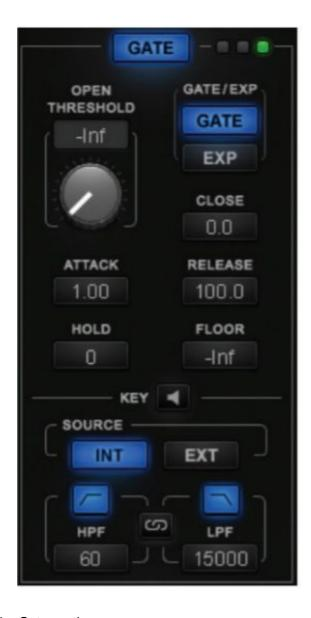
**GATE**: Turns on or bypasses the Gate section.
