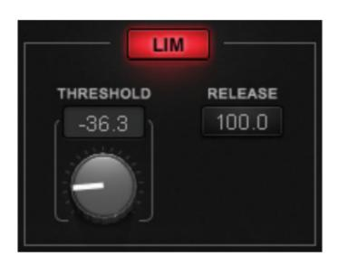
LIM: Turns on or bypasses the Limiter section.
