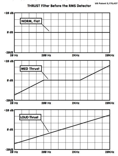
**Type**Sets the Compression type, which determines the signal source being fed to the RMS detector.
