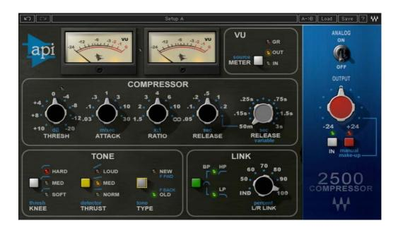
The API 2500 is a versatile dynamics processor that lets you shape the punch and tone of mixes with absolute accuracy. Its dual channel design lets the 2500 also function as two separate mono channels via a single compression setting. Using auto-makeup gain, you can adjust Threshold or Ratio while automatically maintaining
