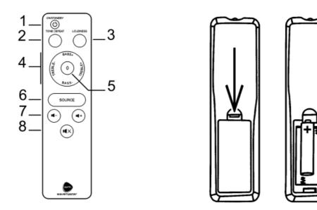
Insert the batteries (2 x AAA batteries) with their polarity according to the markings in the battery compartment. Wrong polarity can cause a defect! With wrong polarity of the batteries, there can be no function of the remote control!
