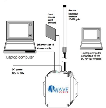
EC-series products are wired into the ship's low voltage supply: 12 volts or 24 volts. Include a line fuse and breaker, and take care with the polarity of the DC wires. The EC unit can also be connected to a 110 volt supply using a switching power supply. Please call Wave WiFi for information.
