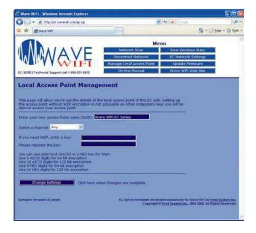
If you had connected to the EC-AP-HP unit wirelessly then your computer wireless card will have disconnected from the EC-AP-HP. Go to the computer wireless configuration screen and look for the new wireless network name that you installed. When the configuration is complete, click on the MENU button NETWORK SCAN at the top of the page.
