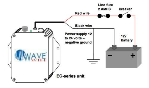
The EC unit is supplied with an LMR-400 antenna cable 25-feet long. This cable should not be substituted with a different type or different length of cable. Substituting the cable supplied may reduce the transmission distance dramatically.
