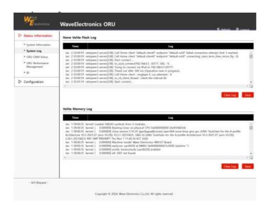
WEH37 ORU supports monitoring system log in non volite/volite areas via syslog. Two red buttons below each log area functions 'clear' or 'save' the log. In case of downloading the log to the PC via "save" button
