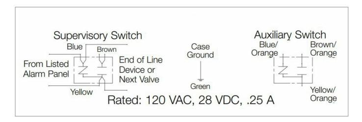
Wire the supervisory switch to a fire alarm control panel in accordance with the schematic diagram. Verify that the switch is operating as intended before commissioning the product. Proper operation must be assured. If adjustment is required to comply with NFPA standards and local ordinances, follow the procedure for switch replacement, starting at step 7. Follow all steps of the field instructions when rotating or replacing the switch.
