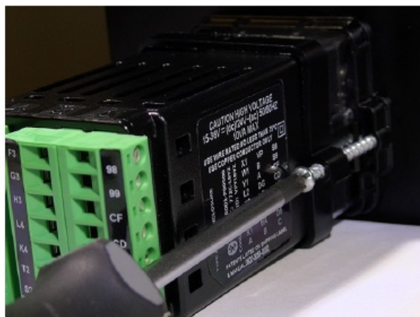
Figure 3: Tighten the Mounting Screws
