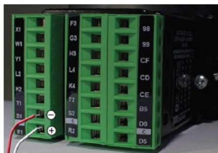
Figure 2: Input Terminal Connection Shown Here
