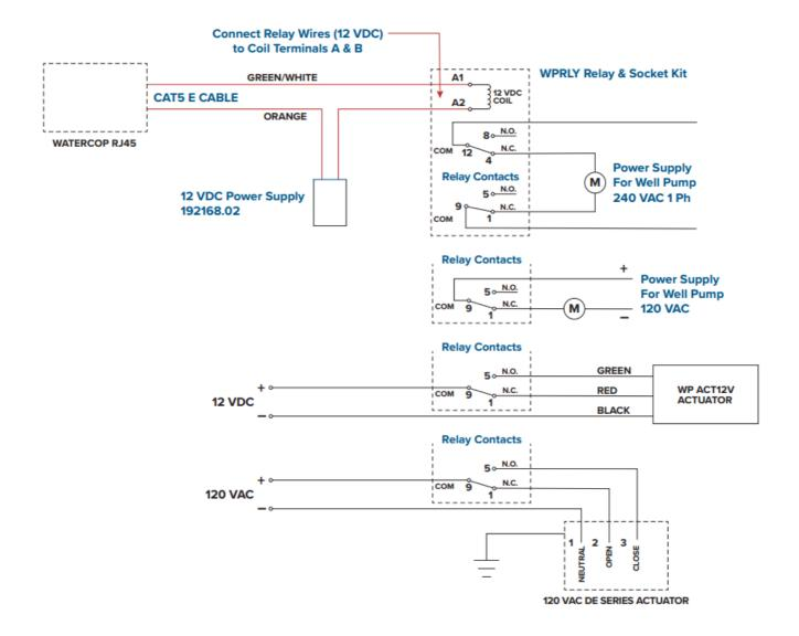
**WARNING!** The relay wire will be energized (12 VDC) when the WaterCop Actuator is powered and is in the closed position. Make connections to the relay coil before energizing the actuator.
